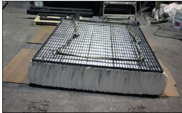
Figure 2. New panel for installation in roof lining of furnaces.
